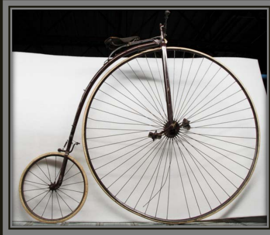
1870 Ordinary, Penny Farthing or High-Wheeler. The large diameter front wheel enabled the bicycle to travel further each revolution, which also increased the bicycles speed.
