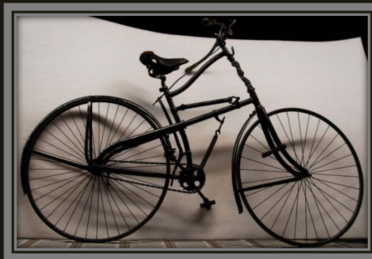
1888 Whippit, with front and rear suspension.
